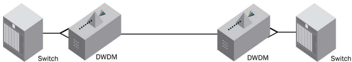
Figure 3. Y-Cable/line card protection
