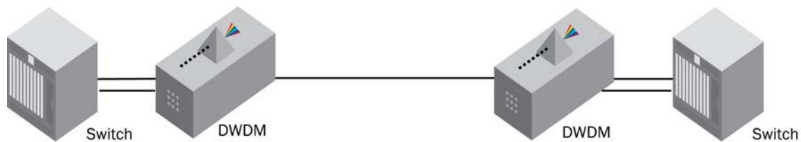
Figure 2. Client-protected topology with multiple ISLs
