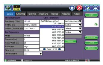
CWDM - Configure with 8/10/18 wavelengths as defined in ITU G.694.2 grid. Simply select via pull down menu.
