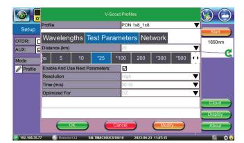
The MTTplus-410+ OTDR employs specialized techniques developed from decades of experience to locate and measure connectors, splices, optical splitters, and macro-bends.
