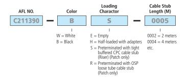
Example: Order number for a panel Black in color, loaded with 72 PSC adapters (12 six packs), connectors and a cable stub 5 meters in length.
