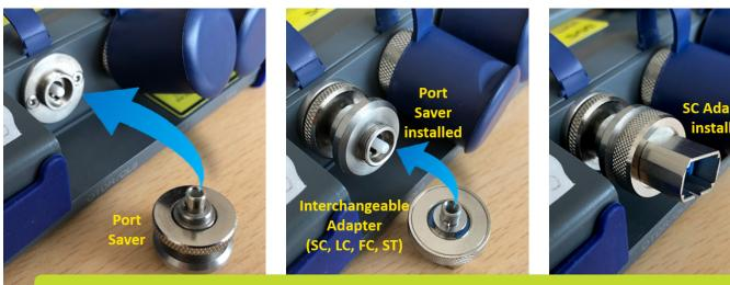
Avoid costly Test Set repairs: Install a field-replaceable port saver!
